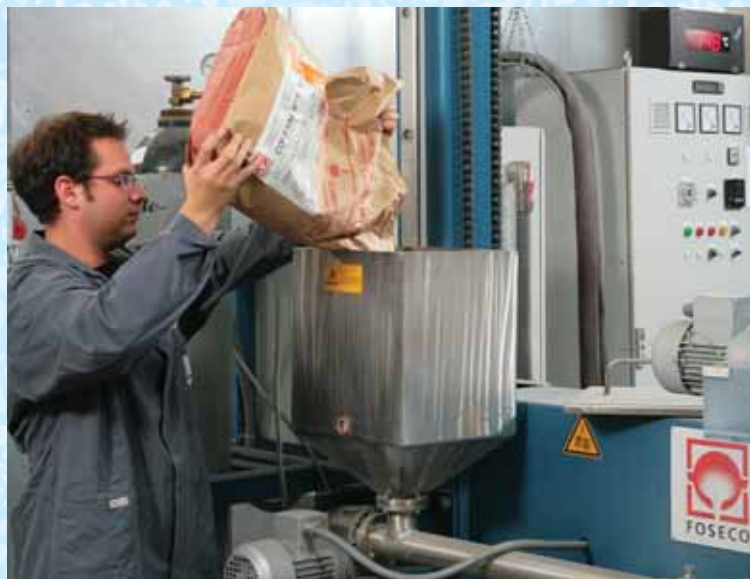
Figure 1 The MTS 1500 automated metal treatment station
