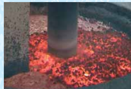
Figure 5 The action of a cleaning flux
