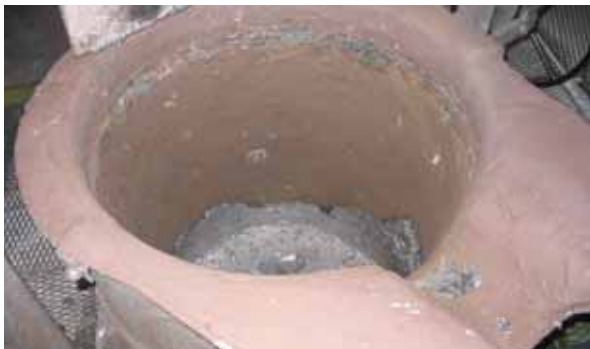
Figure 4 An INSURAL ATL ladle, which has been coated regularly, after 4000 fillings. The metal skull in the base is still easily removed by a gloved hand
