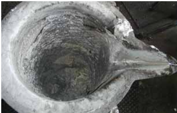
Figure 3 A conventional concrete ladle after 4000 fillings, showing a heavy build up of oxide
