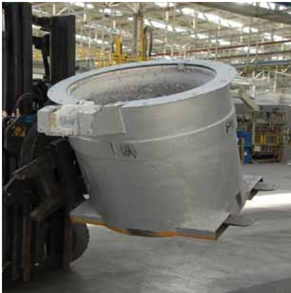
Figure 6 INSURAL ATL1000 IB-Ladle with a capacity of 900kg
