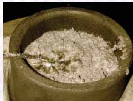
Figure 5 Melt with addition of flux
