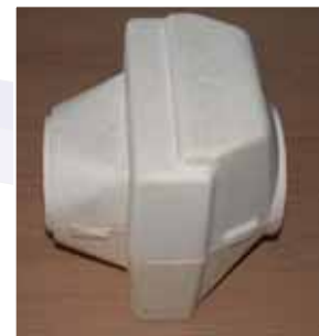
Figure 14 Ceramic print for vertical filter placement
