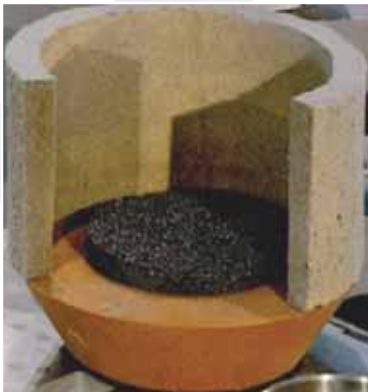
Figure 16 Cylindrical feeder with filter carrier core
