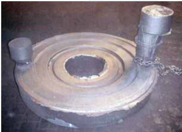
Figure 27 Direct pour through a KALPUR unit
