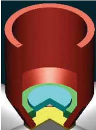
Figure 15 Neck down feeder with insert filter carrier core
