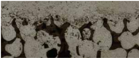
Figure 10 Deep bed filtration
