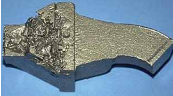
Figure 9 Trapping of large inclusions at the entrance
