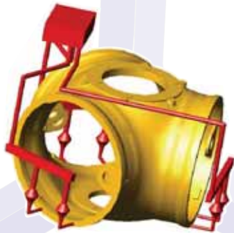
Figure 21b Filters placed in ceramic prints short before the ingates
