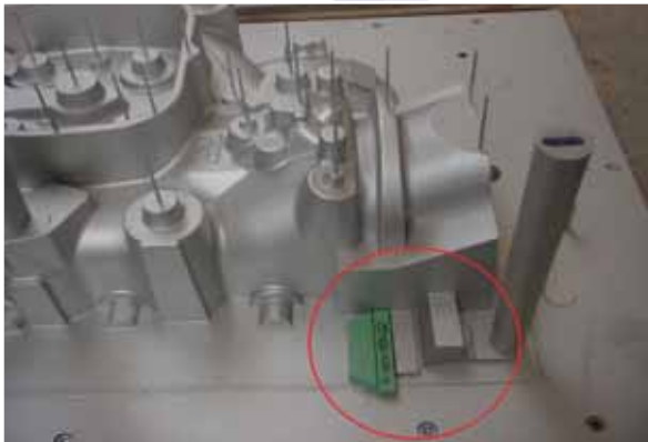
Figure 18 Drag and cope site of the pattern plate
