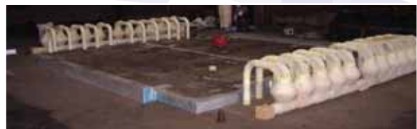
Figure 23b Two rows of 200mm diameter ceramic filter prints are needed to cast a 25,5 t GJS casting
