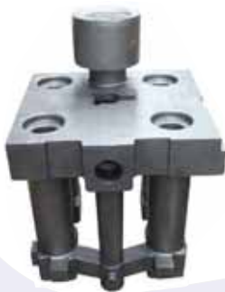
Figure 28 Casting with remaining feeder
