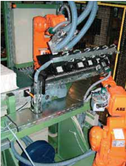
Figure 6 Robotic positioning of SEDEX filters in the core mask
