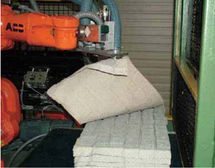
Figure 5 Robot automatically removes protective paper
