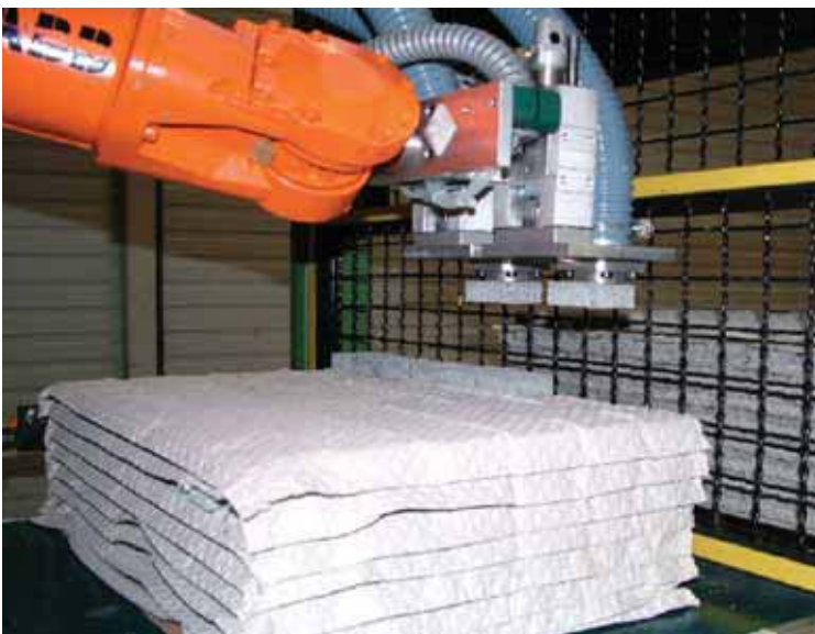
Figure 4 Robotic pick-up of SEDEX filters
