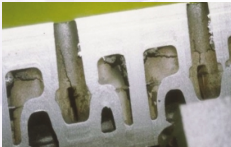
Figure 1 Vein defects in cylinder head
