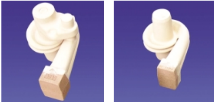
Figure 12 Turbo housing cores dipped in RHEOTEC XL coating
