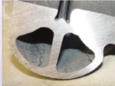
Figure 11 Veining defects prior to the use of RHEOTEC XL coating
