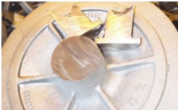
Figure 17 Sectioning of the reverse taper direct pouring stub confirmed soundness of the casting at the point of contact
