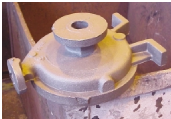
Figure 10 This centrifugal pump body casting was converted to direct pouring using a reverse taper unit
