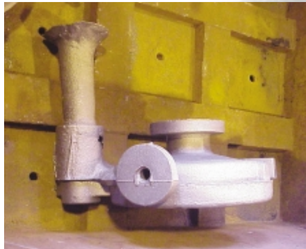
Figure 8 In this side-gated application, the reverse taper unit is mounted on a riser base close to the casting
