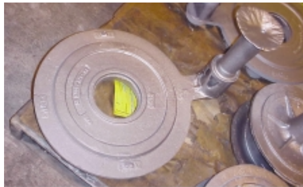
Figure 12 This side-gated iron bearing housing casting is poured through a downsprue positioned above a reverse taper direct pouring unit
