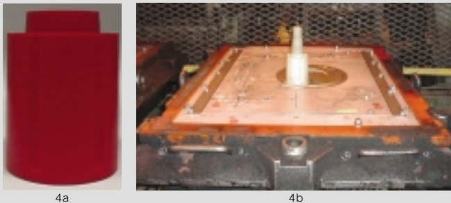
Figure 4 A special riser bob creates a cavity for insertion of the reverse taper unit
