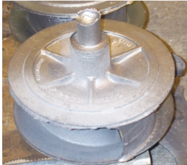
Figure 15 The impeller was cast with a reverse taper direct pour unit that eliminated the need for all conventional gating components*
