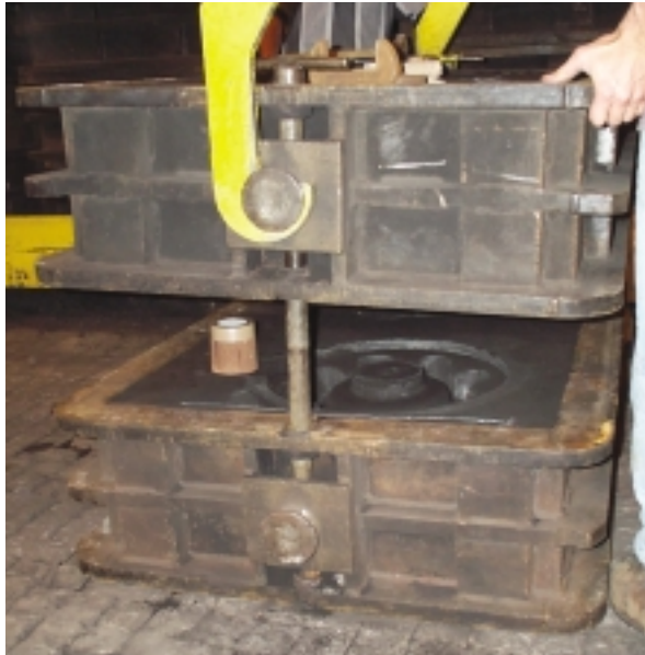
Figure 13 The bearing housing mould is closed over the reverse taper unit
