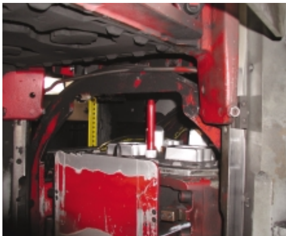
Figure 9 Height limitations on some moulding machines restrict the height of pattern components such as sprues, risers and direct pour units
