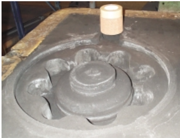
Figure 7 For close-over side feeder applications, the reverse taper unit is positioned in a moulded recess in the drag prior to closing the mould
