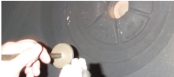
Figure 16 The direct pour unit is easily inserted into the inverted cope half of the impeller mould using a simple insertion tool
