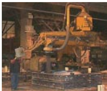
Figure 8 Mould filling of large flasks using continuous mixers
