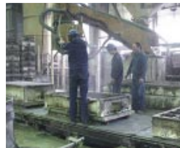
Figure 7 Facing (30%) new sand. Backing (70%) reclaimed sand with continuous mixer in one step
