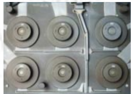
Figure 3 Pattern plate with the first gating system concept
