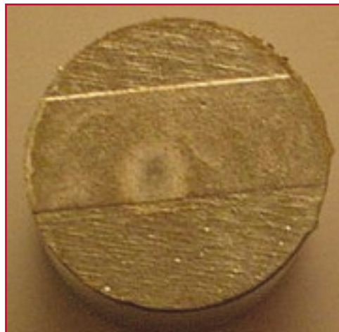
Figure 7: Photograph of a casting made on the "ideal" coating surface shown in Figure 5 showing a central rough patch, corresponding to the point of impact of the metal stream. (The parallel-sided feature on the casting surface shows the region where grooves were machined in the coating of the die steel block)
