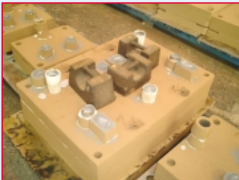
Figure 4: Chassis casting immediately after pouring, showing three KALPUR units
