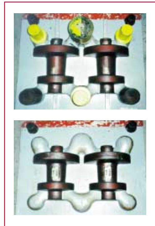
Figure 8: Cope and Drag patterns for 2-up valve body casting
