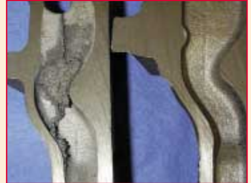
Figure 4. Penetration defect in 1.8ltr engine block oil gallery (left-hand section) eliminated through the use of RHEOTEC XL coating (right-hand section)
