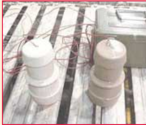
Figure 2: Coated test piece cores
