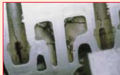
Figure 1: Veining in a sectioned diesel cylinder head casting
