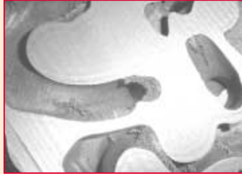
Figure 6: Extensive veining prior to use of RHEOTEC XL coating
