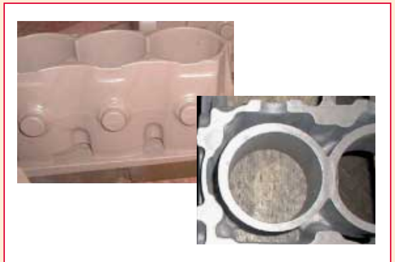
Figure 9: RHEOTEC XL coated water-jacket core and resulting defect free internal finish
