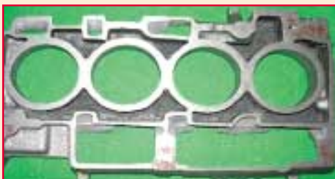
Figure 8: Veining and retained particulate levels prior to use of RHEOTEC XL coatings
