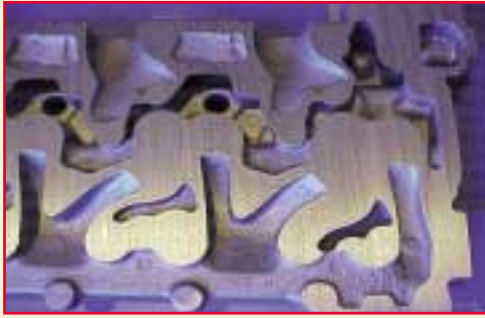
Figure 7: Defect free internal channels when using a single coating application of RHEOTEC XL
