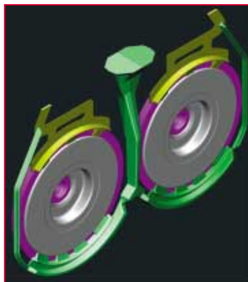
Figure 2: Bottom filled system with 2 cavities
