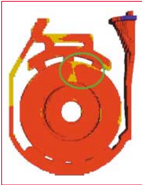
Figure 4: Area of cold metal corresponding to the presence of under-cooled graphite
