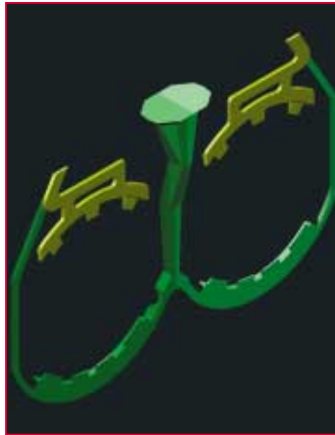
Figure 5: Current running system. The ingate and flow-off are in the same plane
