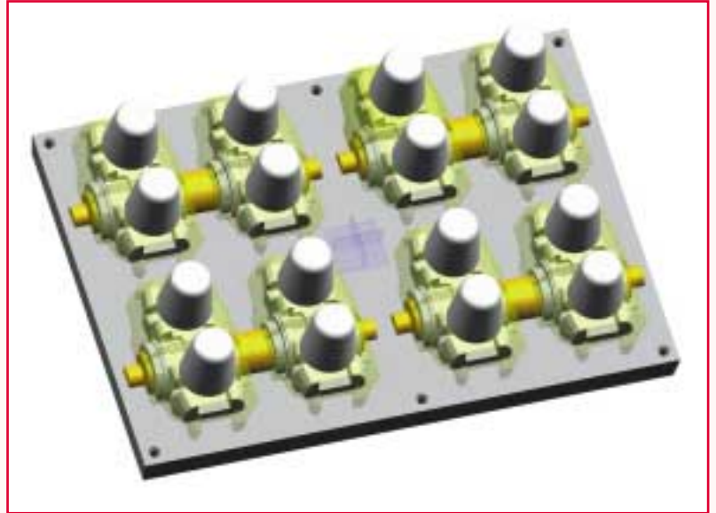
Figure 5: Casting example 1 using traditional sand feeders
