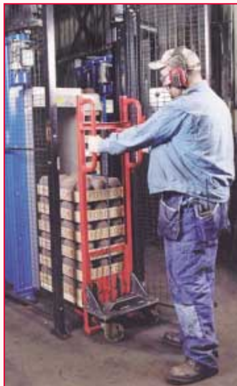
Figure 3: Forklift device with trays to be loaded into a sleeve magazine
