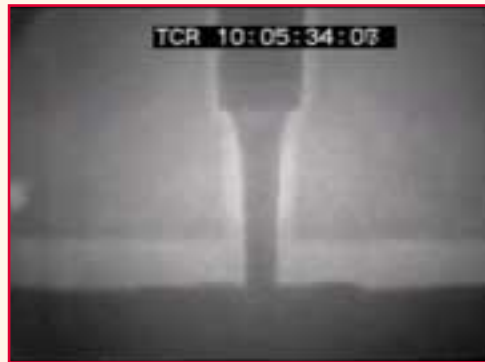
Figure 2b: Top-gated plate-mould real-time X-ray, ceramic foam filter in direct pour sleeve
