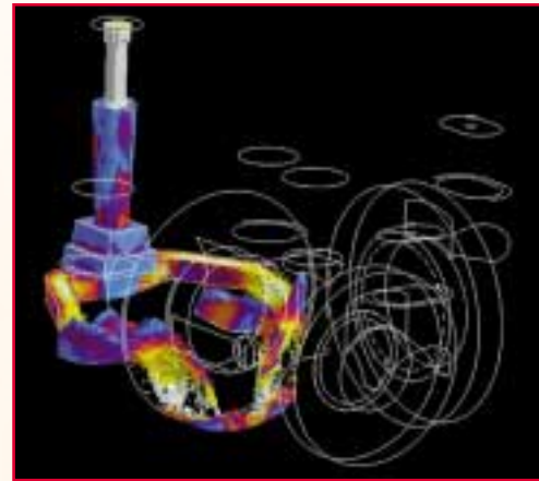
Figure 7: Simulation of metal flow in conventionally gated valve casting with zirconia-based ceramic foam filter positioned at base of downsprue
