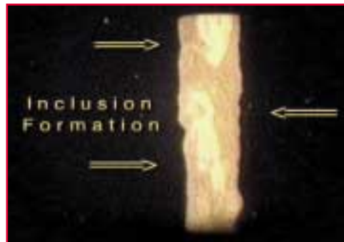
Figure 10: High speed video showing formation of reoxidation inclusions
