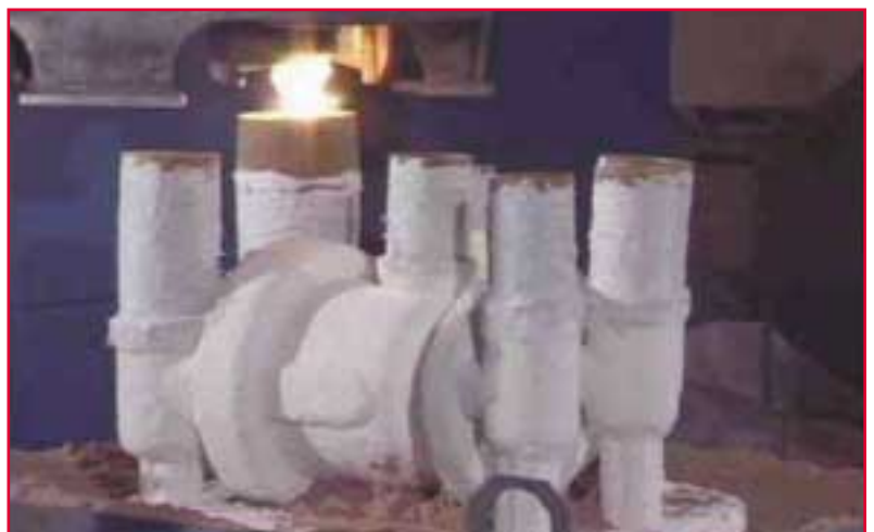
Figure 20: Specialized shell mould used to facilitate x-ray visualization of valve casting during pouring
