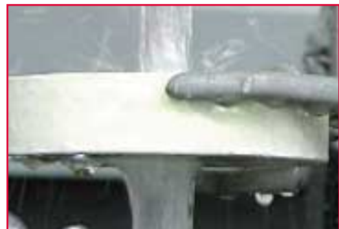
Figure 2: Stream of water passing through strainer core shows little reduction of turbulence
