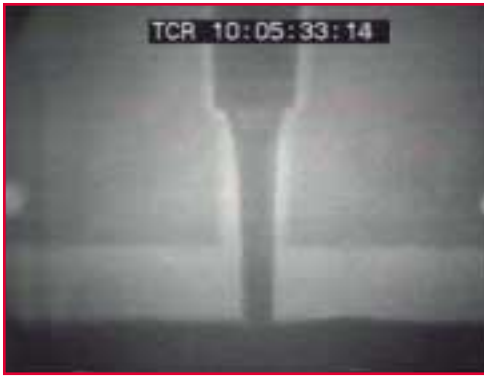
Figure 14: X-ray view of filtered top-gated plate casting showing reduced turbulence as metal enters casting
