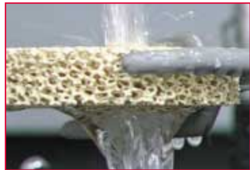
Figure 1: Ceramic foam filter reduces turbulence from stream of water
