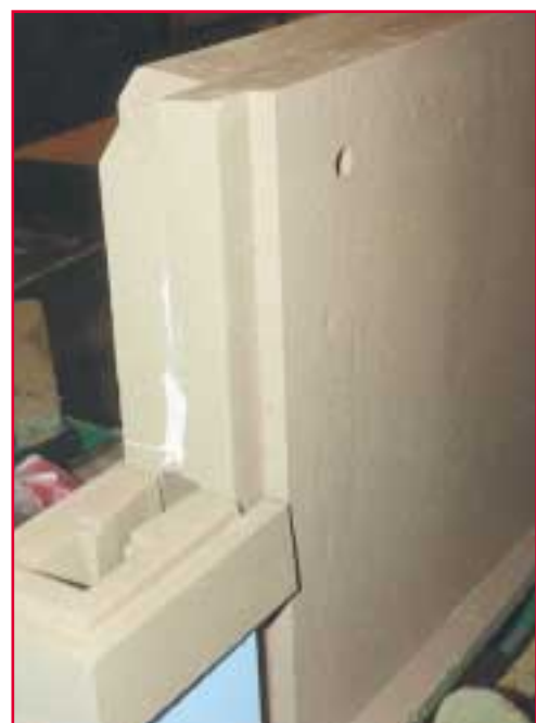
Figure 9: Plate mould supported in steel frame for x-ray trial
