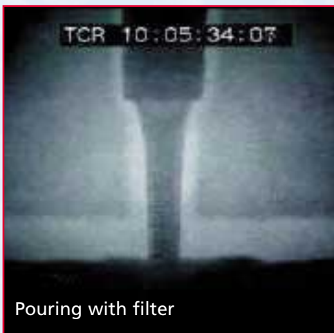
Figure 12: X-ray analysis shows the ability of filtration to reduce turbulence in molten metal entering the casting cavity
