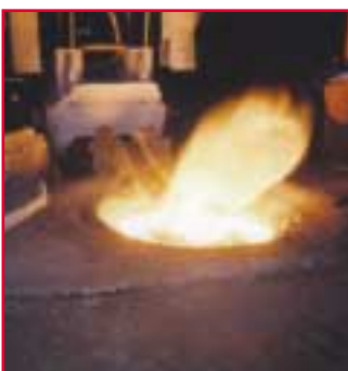
Figure 13: Raw perlite dusting for slag agglomeration
