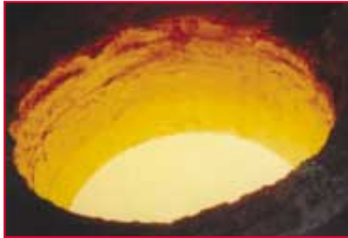
Figure 18: Furnace level of 22 tonnes ready for a second tapping. note the cleanliness of the bath and the lining
