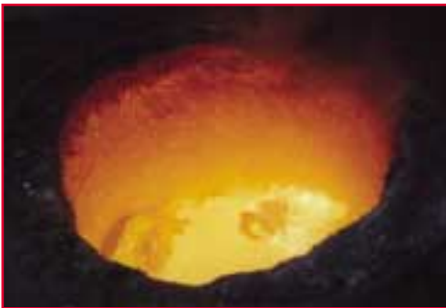
Figure 11: Sandwich additions between two metal charges
