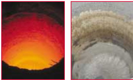
Figure 19 View of an empty crucible after a 4 week campaign and over 2000 tonnes of molten metal. Average diameter 1485 mm, depth 2780 mm. The wall is smooth and only shows a slight elephant foot formation at the bottom of the furnace.
