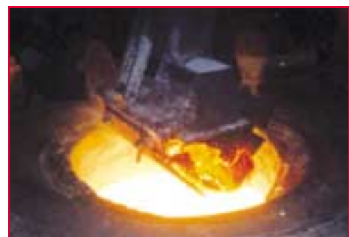
Figure 17: The consistency and compactness of the slag facilitate its removal
