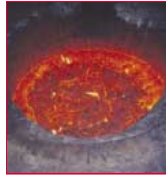
Figure 14: Slag film floating on the top of the bath after a few minutes of decantation
