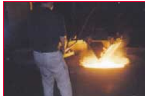
Figure 16: Mechanical slag extraction
