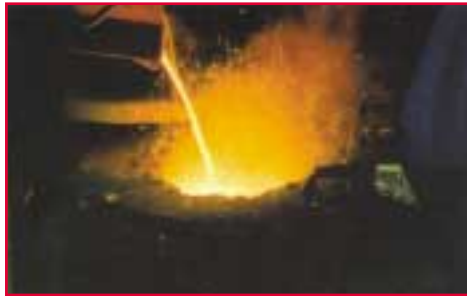
Figure 2: Typical spark emission of an oxidised melt during decanting from ladle into a furnace
