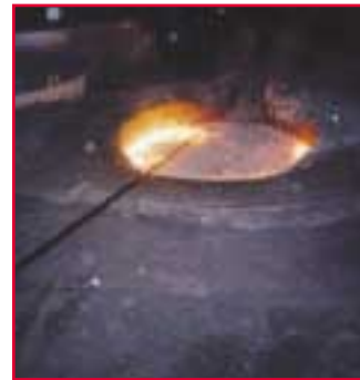
Figure 15: Slag removal from the furnace wall
