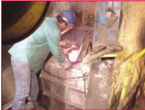
Figure 21: The operator adds pure Mg and 10g of FERROGEN 8 per tonne of treated iron.
