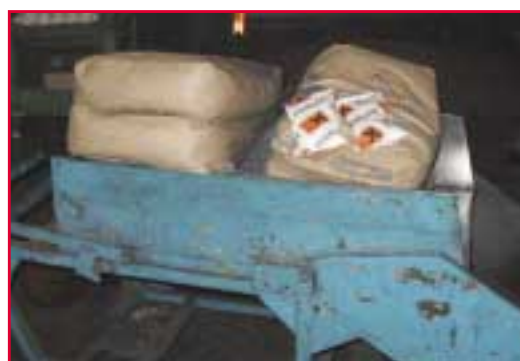
Figure 9: Additions : Graphite, SiC, Ferrogen 8 for a metal charge of 6 tonnes
