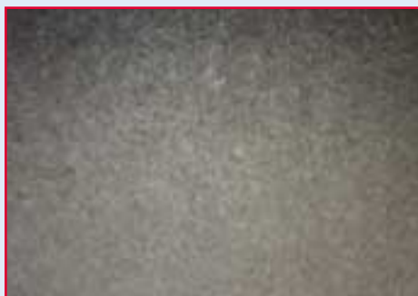
Figure 5: Smooth stabilised surface at high temperature on coated greensand core
