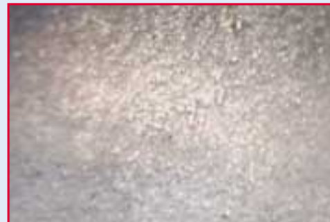
Figure 8: Point 'B' – casting produced using a Coated Mould
