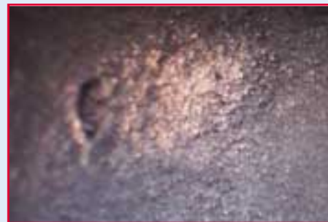
Figure 7: Point 'A' – casting produced using an un-coated Mould
