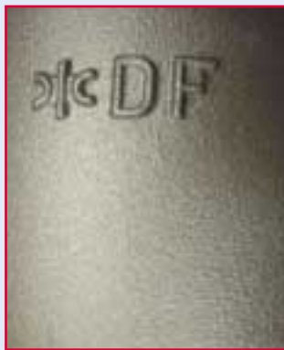
Figure 12: Casting surface from Coated Mould
