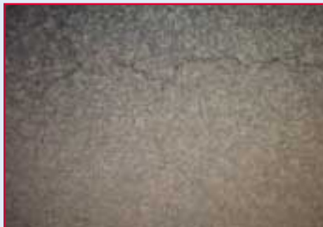
Figure 4: Cracking at high temperature on un-coated greensand core
