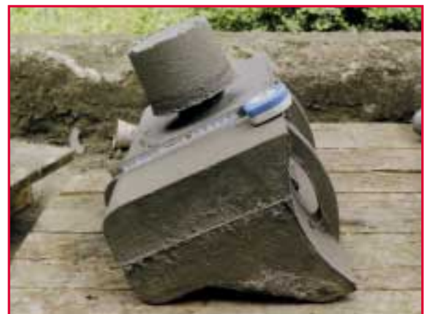
Figure 10: Side view of the casting with the riser.
