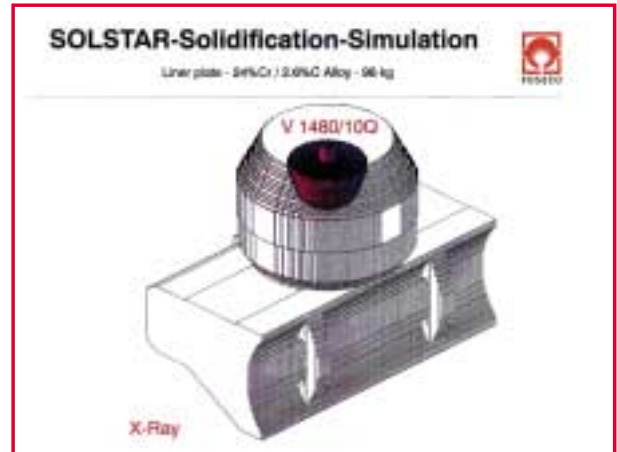
Figure 8: SOLSTAR X-ray Analysis of the casting. The shrinkage is located on the top of the riser, entire casting is otherwise sound.
