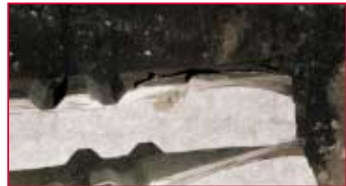
Figure 4: The casting with the knocked-off riser. In the riser casting interface, shrinkage cavity can be seen, otherwise the casting is sound.
