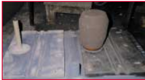
Figure 1: Two castings on the pattern plate; on the left-hand side the requisite pattern for a FEEDEX HDV 780/10 Q and on the right-hand side, the feeder sleeve already located on the pattern plate.
