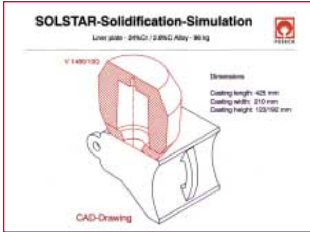
Figure 5: CAD drawing section through the casting and casting dimensions.
