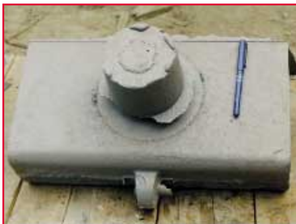
Figure 9: The actual casting lengthways with the riser.
