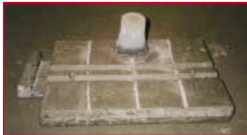
Figure 3: The casting with the riser.
