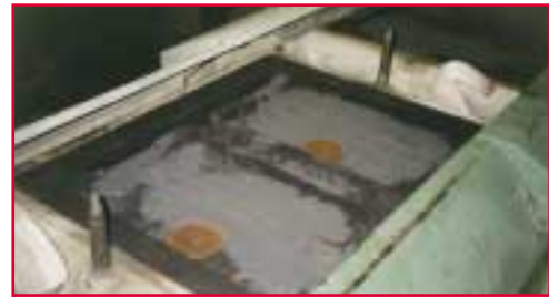
Figure 2: The mould turned over where breaker cores can be seen.
