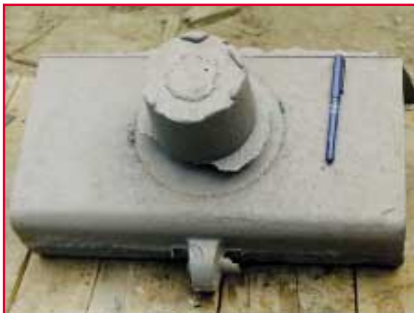
Figure 9: The actual casting lengthways with the riser.
