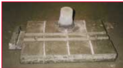
Figure 3: The casting with the riser.
