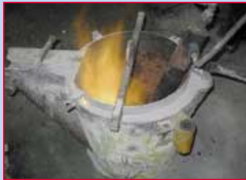
Figure 5: A gas flame is applied to initiate the exothermic reaction
