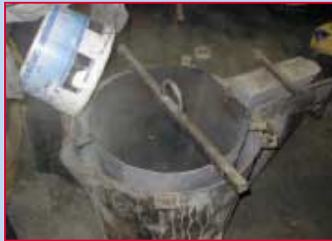
Figure 3: The dry KALTEK ISO powder is poured between the ladle shell and the former
