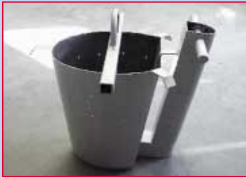
Figure 2: A former for the production of a T-Pot ladle, this is stripped from the ladle in 3 parts
