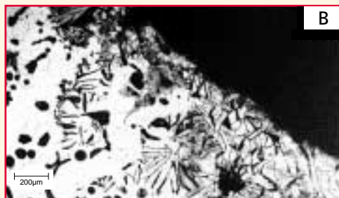
Figure 4b: Casting structure using coating B
