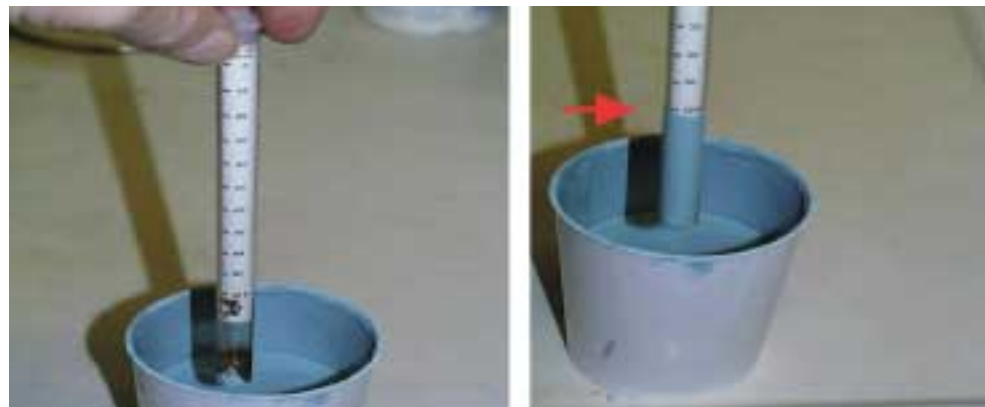
Figure 3: Measurement of Baumé with a Baumé Stick
