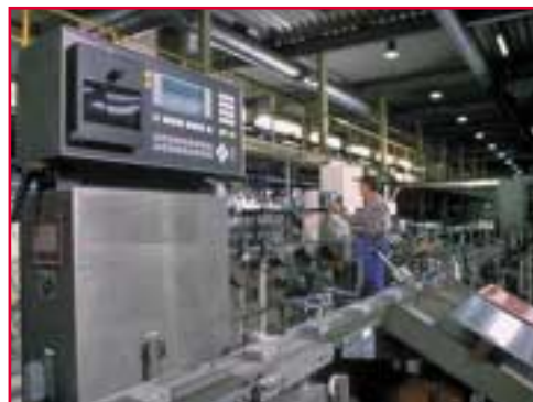
Figure 5: Filter weighing equipment, integrated into the production line.
