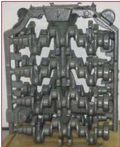
Figure 14: Eight casting spray viewed from the other side.
