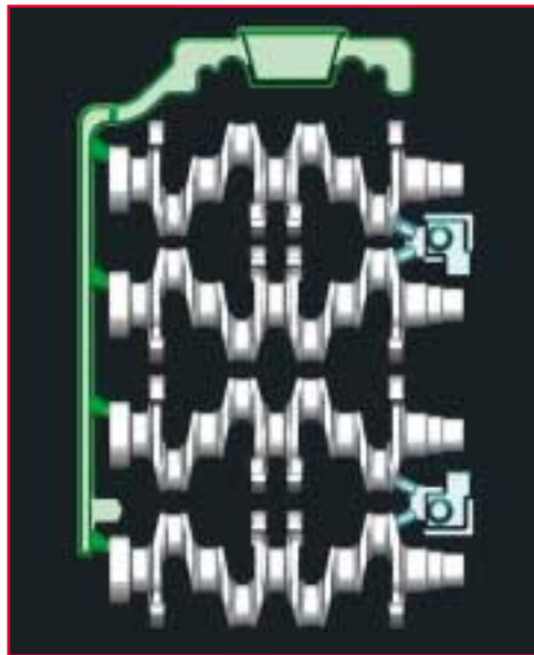
Figure 15: One half of the 3D virtual spray used for the mould fill simulation shown overleaf.
