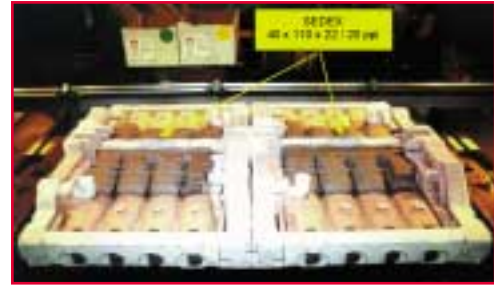
Figure 25: Open four cylinder block mould.
