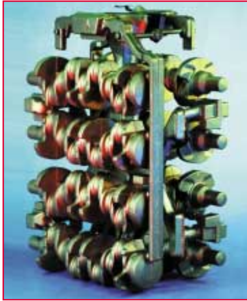
Figure 12: Eight casting layout, actual spray still in the same box size.
