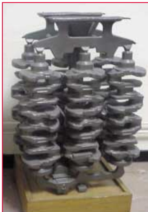
Figure 10: Spray of 6 castings, poured weight 120kg.
