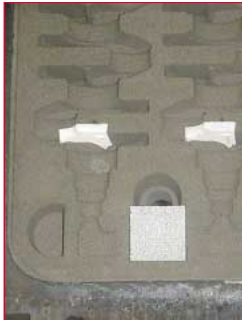
Figure 11: Open sand mould with single filter for 3 of the 6 crankshafts.
