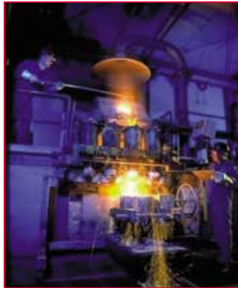
Figure 2b: Impingement testing in progress with liquid iron.
