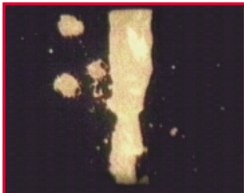
Figure 9 - Slow Motion Videography of the metal stream exiting a bottom pour ladle. Inclusions can be seen forming on the surface of the metal stream
