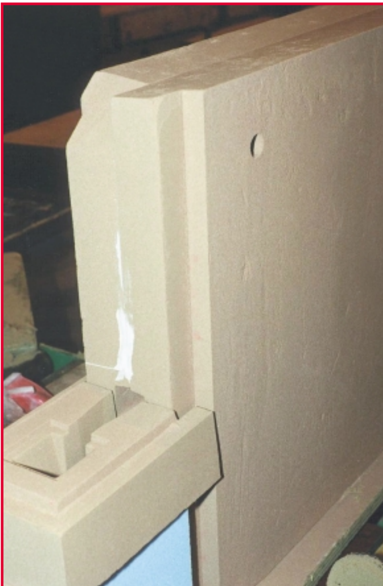
Figure 6 - A mould being fabricated showing a filter print in the running system
