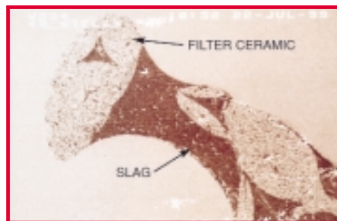
Figure 4 - A Scanning Electron Micrograph of slag adhering to the surface of a used STELEX filter
