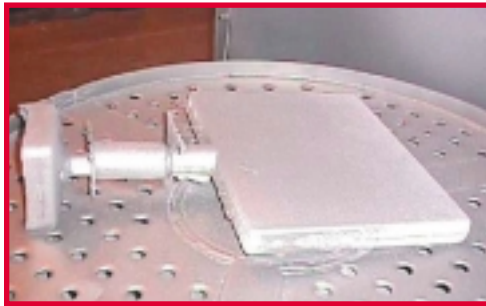
Figure 16 - The resultant casting from one of the tests
