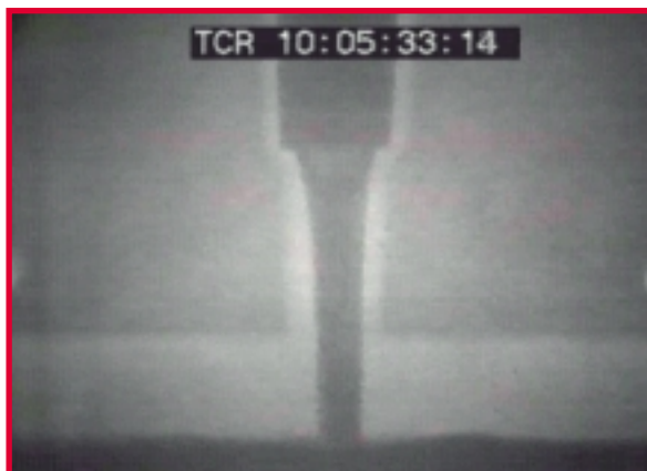
Figure 13 - With the KALPUR applied to the top gated mould a controlled metal stream exited the filter resulting in a non turbulent fill of the casting cavity
