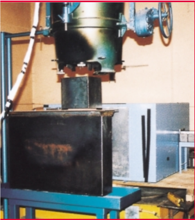
Figure 8 - The ladle over the mould in the X-ray bunker
