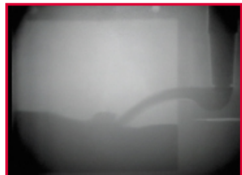
Figure 15 - Application of a filter system to the side gated mould resulted in a Non turbulent mould fill
