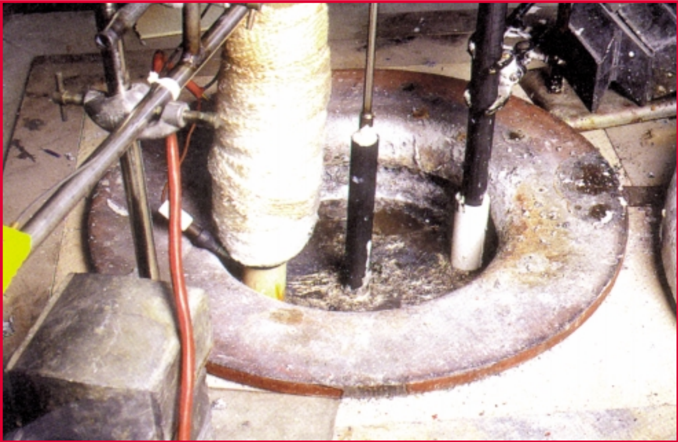
Figure 4 - Original COSMA concept under foundry test
