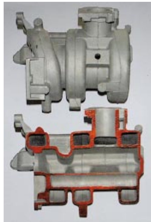
Figure 2: This aluminium intake manifold for a three cylinder engine with its thin 3mm walls, cast in holes and narrow 4mm diameter air channel gave the foundry a 15% weight reduction and 30% cost reduction. (Courtesy of Alluminio Dongo SpA, CAGIVA Group).
