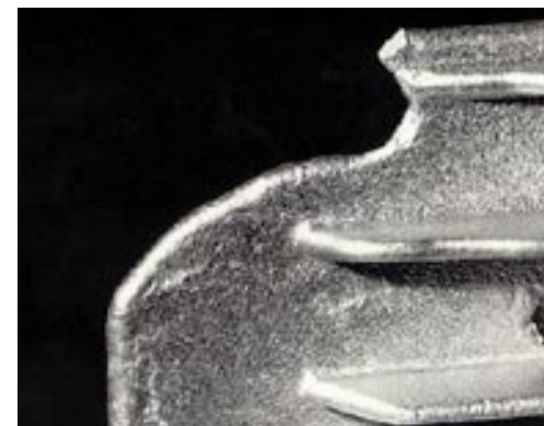
Figure 7: An example of a mis-run defect caused by the use of a coating with insufficient permeability or thermal insulation.
