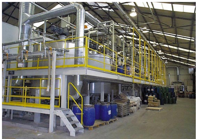
Figure 9: The SMC Netherlands state of the art computerised coatings plant is used to manufacture high quality foundry products, including the SEMCO PERM and STYROMOL lost foam coatings.
