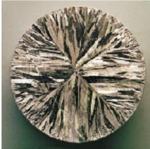
Figure 5a: Pure aluminium 99,7; unrefined.
