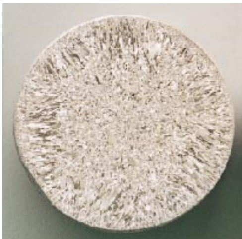
Figure 5b: Grain refinement by addition of 0,05 % NUCLEANT GRI 2850.
