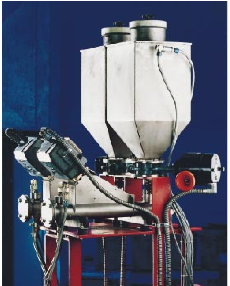
Figure 3: Dosing device of the twin injector.
