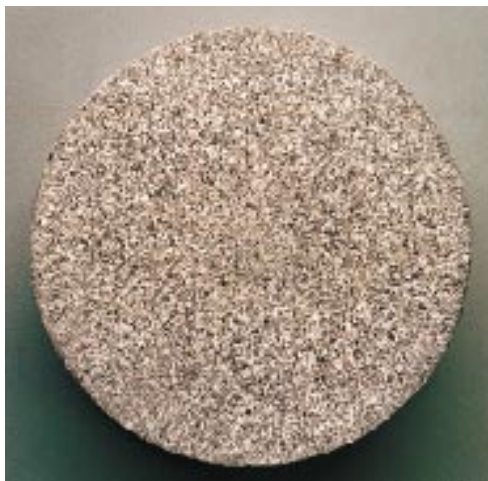
Figure 5c: Grain refinement by addition of 0,08 % NUCLEANT GRI 2850.
