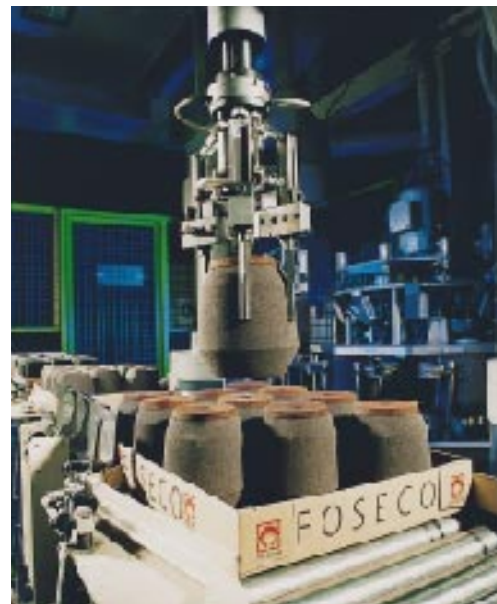
Figure 6 :Automatic gluing of breaker cores to VS sleeves.
