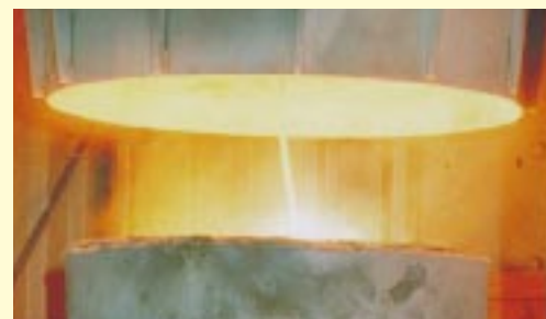
Figure 6: View into a treatment station. 1600 kg treatment weight 9 mm IMPREX 8/9 (pure Mg cored wire).
