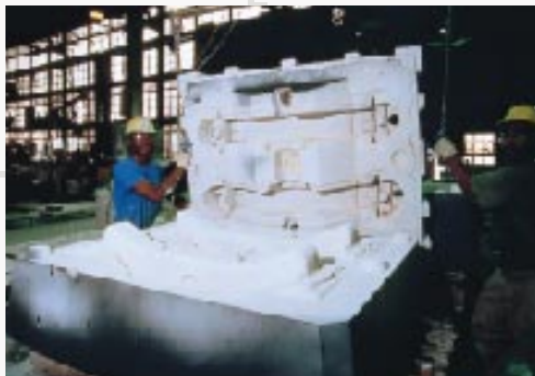
Figure 2: No-bake mold optimized with Foseco feeding systems
