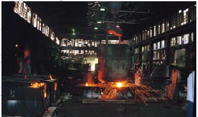
Figure 4: Bottom pouring in large bay
