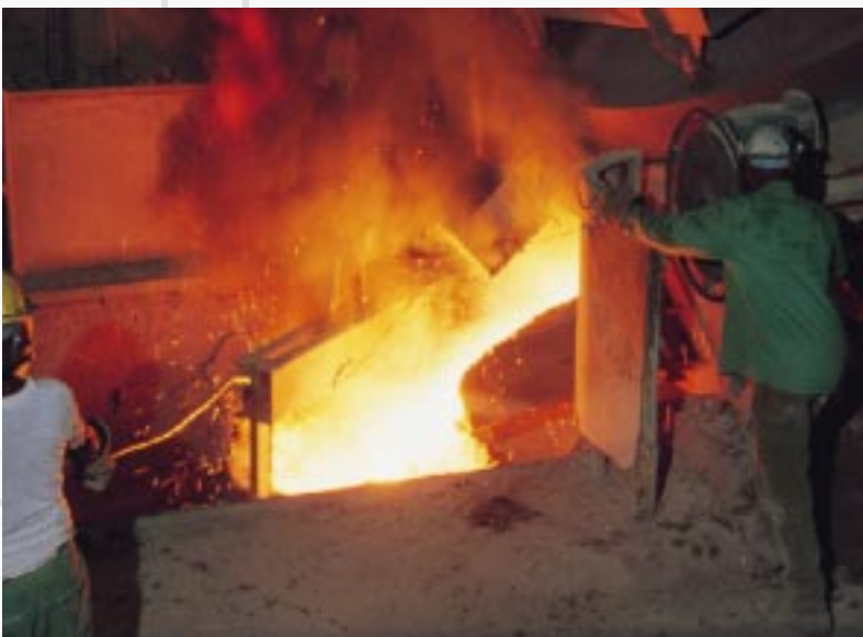
Figure 1: Tapping the electric arc furnace
