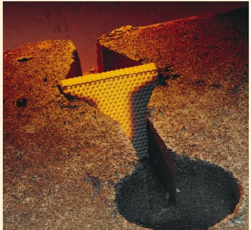
Figure 5: New triangular-cell extruded ceramic filter prior to pour
