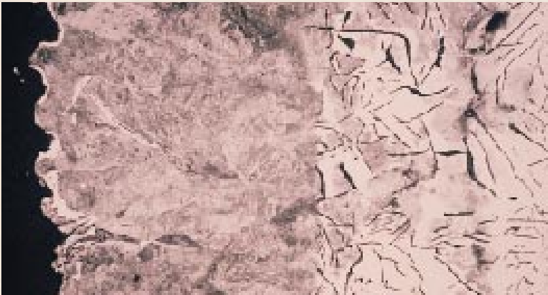
Figure 2: Graphite free rim in a pearlitic grey iron
