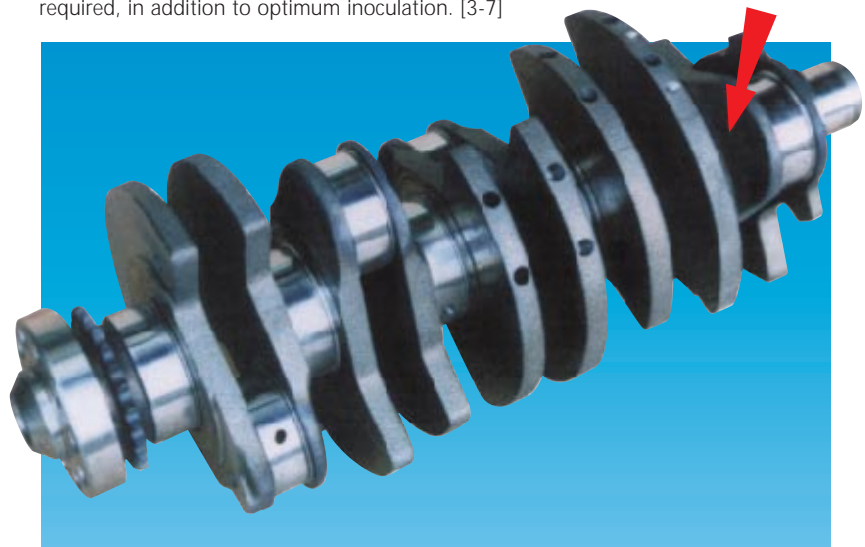
Figure 1: Machined VR crankshaft. The arrow illustrates the defect position in counter weight 2
