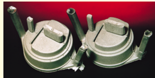
Two filter support gravity die castings after shot blasting showing how use of a SIVEX FC filter in the downsprue reduces the effects of turbulence.
