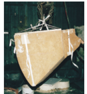
Figure 6: The pre-assembled KALTEK ladle lining system
