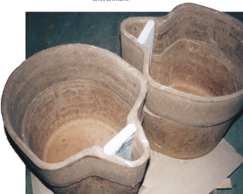
Figure 3: 1,100 kg capacity teapot KALTEK ladle
