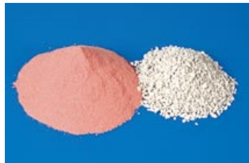
Granular flux compared to conventional powder flux.
