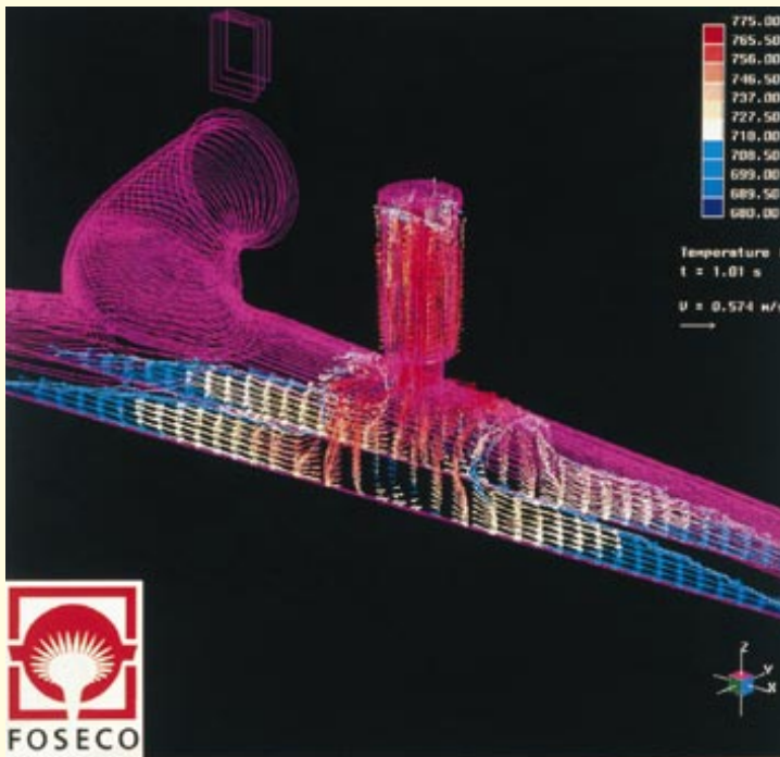
Figure 3: Air inlet manifold showing flow simulation study.
