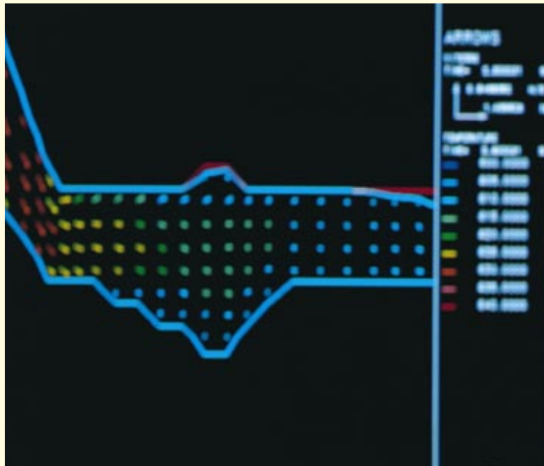
Figure 6: Flow simulation through a foam filter.
