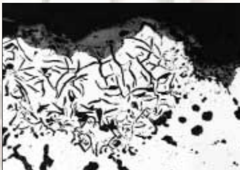
Figure 6. Light microscope photo micrograph of the edge zone of sample 70 with very pronounced surface defects (master alloy FSM 2, mould inoculation with IM 9).
