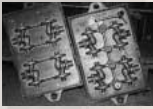
Figure 1 Pattern plate of the test casting (valve body).
